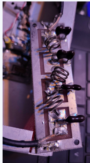
FIG 4 — 7-element Chebyshev LPF. Three bare-wire air-core coils (5T #18, 1/4" dia) with four 27 pF black ceramic shunt caps.
